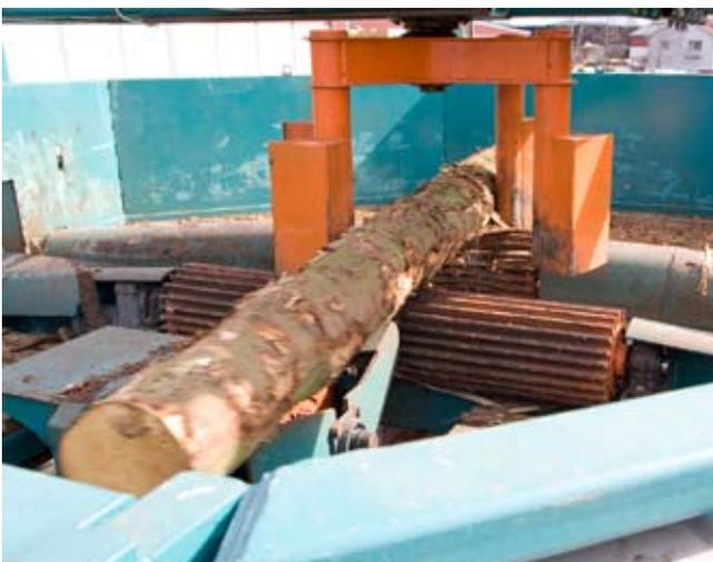
*The logs pass through a proving frame which checks that the narrower top end is coming out first. The logs lying with the butt end first are turned around in a log turner.*
