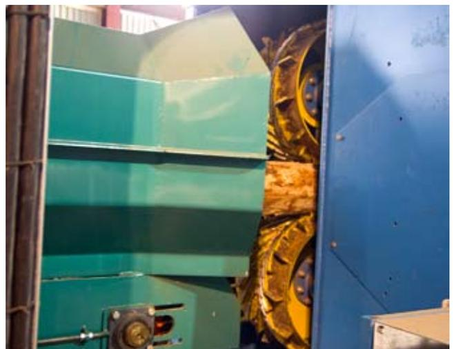
*Fast deceleration saves valuable time. An Emotron FDU variable speed drive with a brake resistor stops the log feed in around one second. Rotors controlled with Emotron MSF softstarters decelerate to a standstill in around 30 seconds.*
