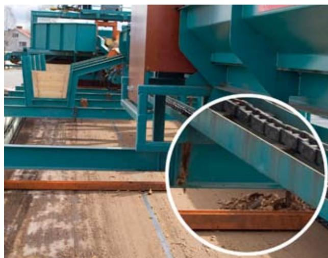
*Underneath the conveyor are chain-driven scrapers which remove muck. Emotron M20 shaft power monitors stop the scrapers immediately if they jam, thus preventing expensive chain breakages.*
